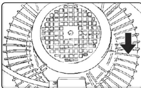
If the direction of rotation is not correct, insert a screwdriver into the notch inside the plug and reverse the two poles with a rotation of 180°.
