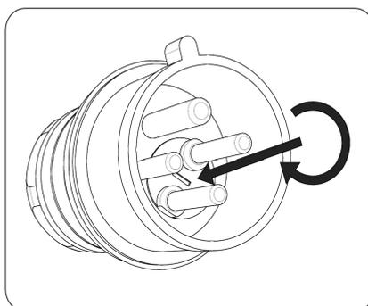
To make sure the vacuum cleaner operation has been properly restored, in addition to checking to make sure it aspirates the air, ensure the pump direction of rotation matches the figure below
