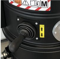
On one side of the filter chamber there is an ergonomic manual shaker through which the operator can easily and quickly clean the filter, removing any dust and debris from its surface. Thanks to this smart cleaning system the operator can carry on working without needing to change or wash the filter.
