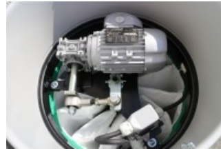
SE Semiautomatic electrical filter shaker
