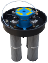
SP Automatic reverse jet cleaning system Antistatic M class filter (EN 60335-2-69), 4 Polyester filter cartridges, 18 m 2 filter surface
