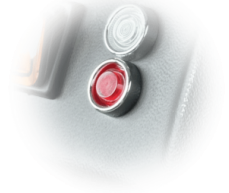
FILTER CLOGGING INDICATOR Filter clogged or need to be replaced indicator light
