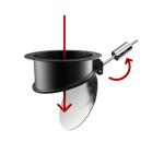
DISCHARGE WITH COUNTERBALANCED FLAP The material is automatically discharged every time suction is stopped.
