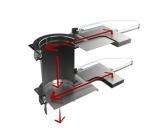
DOUBLE DISCHARGE WITH ELECTRO-PNEUMATIC DAMPERS
