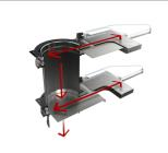
DOUBLE DISCHARGE WITH ELECTRO-PNEUMATIC DAMPERS System with dampers that open alternately to allow the material to be discharged and the vacuum to be maintained at the same time.
