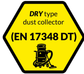
DRY TYPE VACUUM CLEANER Atex-certified vacuum cleaner with dry dust filtration, as per EN17348
