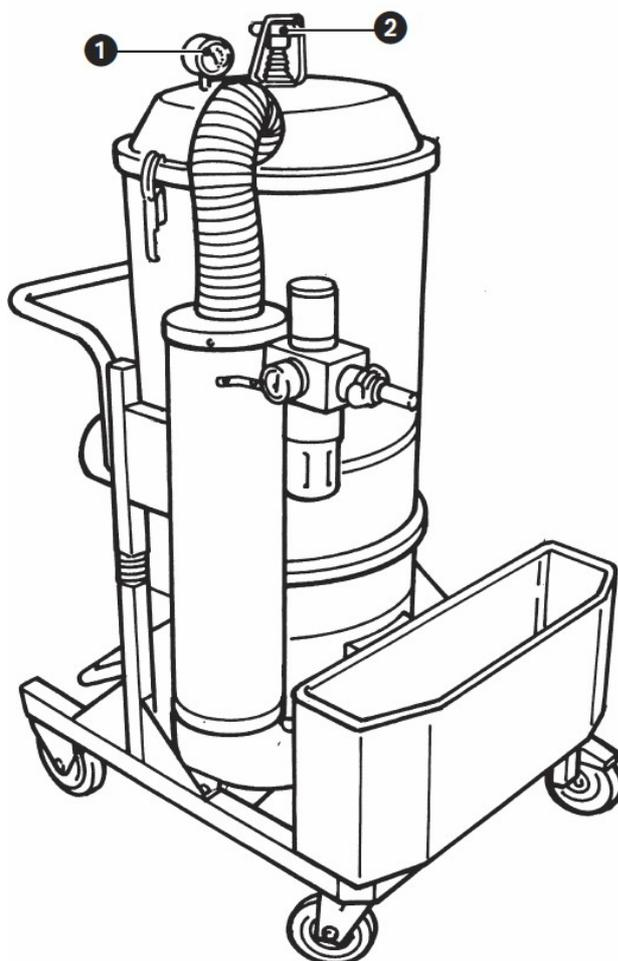
1. Pressure Gauge: indicates filter clogging
