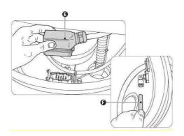
Remove the filter (complete with support and piston) and place it gently on a workbench
