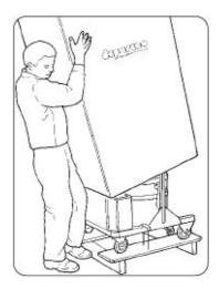
loosen and remove the fastening screws and brackets from both sides
