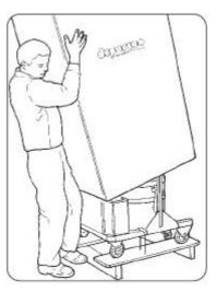
Cut tapes between the platform and base of vacuum cleaner
