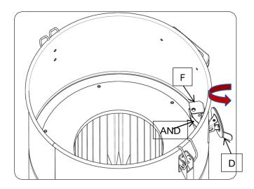
Unscrew the fastening screws of the filter cartridge and pull it out from inside the filter chamber.
