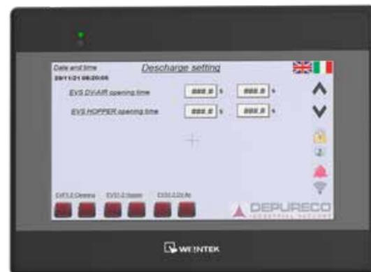
Customize the settings for the automatic material discharge system according to your needs, with extreme ease.
