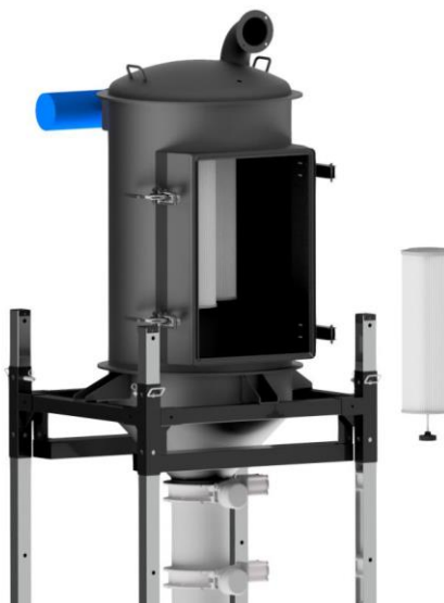
Supporting rod extraction and filtering cartridge replacement
