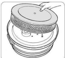
Install the new filter and lock all with the (A) previously removed screw.
