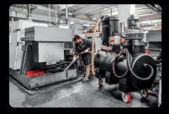
Fast removal of swarf, debris and
