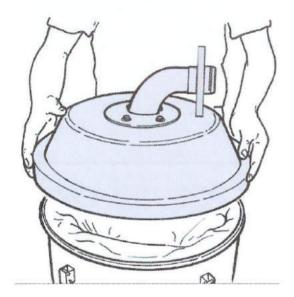
In the event of debris inside the filter or perforated filter, lift the filtering unit from the handles, remove the filter and clean the filter holder.
