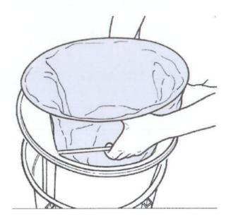
Rinse the filter holder, insert the new filter and reassemble everything inside the compartment, placing the cover back on and locking it.
