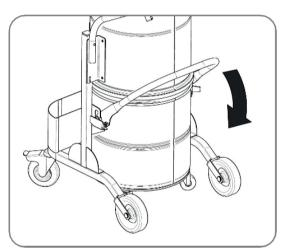
Lower the container lock lever completely and with both hands.
