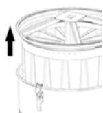
• Loosen the "H" fastening clip, remove the filter from its support and, using scissors, cut the lower belts that clamp it to the filter's cage.
