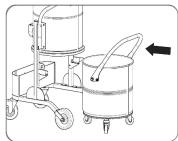
• Check that the pins (A) on both sides of the container are aligned with the slots (B) of the guides.
