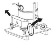
Remove the machine from the support platform by helping yourself with a ramp of suitable capacity and leading the vacuum from the handle.
