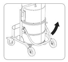
Pull the container (Part.5 Page 9) out from under the chamber.
