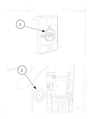
General switch 1 ON-OFF 2. vacuum meter FILTER CLOGGING
