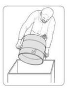
• In case of using a plastic bag for debris collection., after removing the container, tie the bag, pull it out and insert a new bag.
