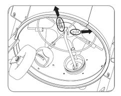
• Release from both sides the two closing hooks (C) of the lid on the filter chamber.
