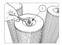
• Slide out and replace the filter cartridges.
