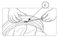
• Using scissors, cut the tapes on the bottom of the filter that secure it to the cage.
