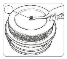
• Remove the filter from the HEPA filter chamber.
