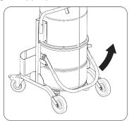
Pull the container (Part.4 section 1.2) out from under the chamber.
