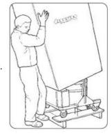
Remove all fasteners provided by the manufacturer at packing stage using appropriate tools.
