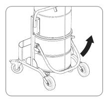
• Remove the container (Part.4 section 1.2) from under the chamber and take it to the designated site for collection/disposal of the inert liquid.
