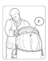
• Loosen the retaining clamp (H) and detach the filter from its holder.
