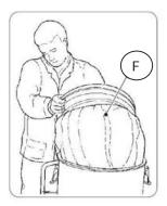
• Loosen the retaining clamp (H) and detach the filter from its holder.
