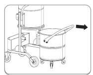
Empty the container into the receptacle intended for waste disposal in accordance with the laws of the country of usea.
