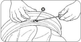
Remove the filter, put it in a plastic bag, close it and dispose of it according to the laws in force for the type of material vacuumed
