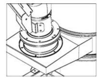
Insert the appropriate accessory for the type of vacuuming from the opposite side of the hose
