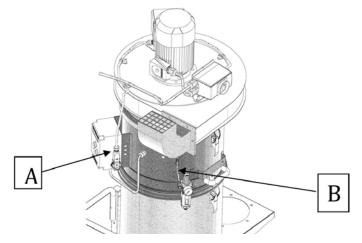
• Unlock the "C" hooks on the sides of the head base on the filter chamber.
