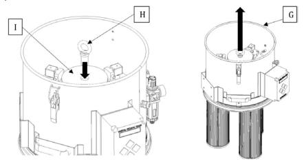
• Remove and unscrew the nuts from the base of the cartridges.
