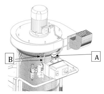
• Unlock the "C" hooks on the sides of the head base on the filter chamber.
