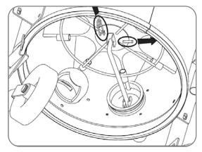
• Unlock the "C" hooks on the sides of the head base on the filter chamber.
