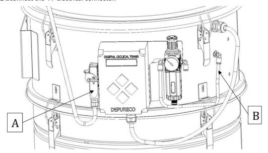
• Unlock the "C" hooks on the sides of the head base on the filter pre-chamber.
