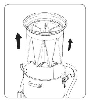
• Loosen the "H" fastening clip, remove the filter from its support and, using scissors, cut the lower belts that clamp it to the filter's cage.
