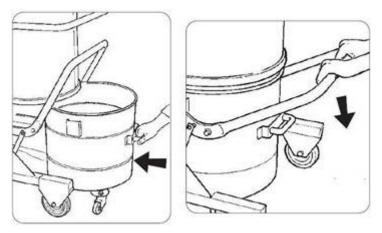
• The "A" pins on both sides must be aligned with "B" the slots.
