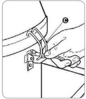
• To lift the vacuum cleaner head, use 3 M8 "E" eye nuts (not supplied) by screwing them onto the pivots of the fan's upper flange.
