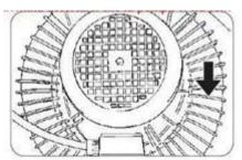
• Turn the switch from I to O [1] to stop vacuuming.
