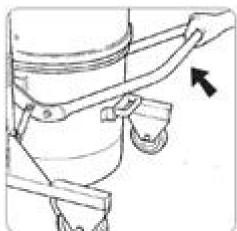
• Remove the container under the filter chamber using the handle.
