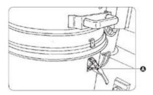
• Using an "H" eye bolt (not included in the supply) with GAS threading and a male G1 connection (screw the eye bolt into the threaded hole on the upper face of the "I" tank) and with the aid of appropriate equipment (straps and lifting and handling systems), lift the "G" filter cartridge support assembly and place it upside down on a workbench.
