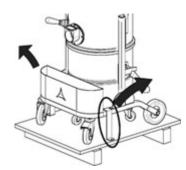
Remove the machine from the support platform with the help of a ramp of suitable capacity and guide the vacuum cleaner using the handle.
