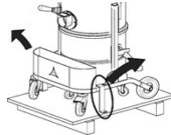
Remove the machine from the support platform by helping yourself with a ramp of suitable capacity and leading the vacuum from the handle.
