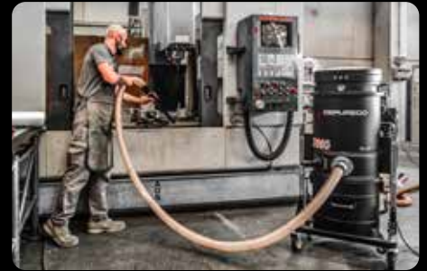
Metal chips cleaning from a CNC machine
